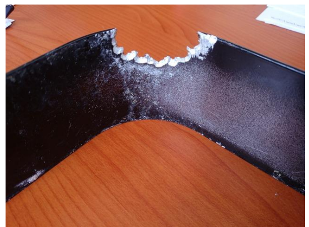
3mm steel kick plate that a rat gnawed through to gain access to food.
